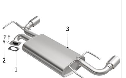
(Carefully read all instructions before installation) Disconnect the vehicle's battery before removal of the OEM exhaust system. This will prevent electrical accidents and will reset the computer if it applies to the vehicle. Remove existing front pipe from the vehicle. Only remove parts that will be replaced. Clean existing flange with a wire brush to ensure proper sealing.
